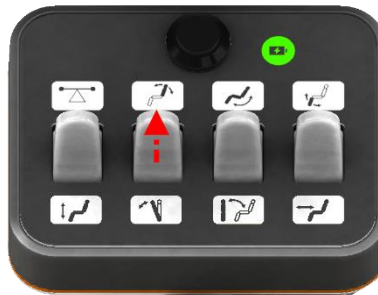
Figure 6-9: Power Recline and Seat Forward Switches – Alternate Between the Switches to Return from Lying Down
